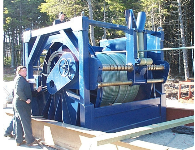
Hawboldt Employees spool customer's cable onto the winch using a large traction winch to provide the necessary tension. Full factory load testing was carried out under DNV survey.
